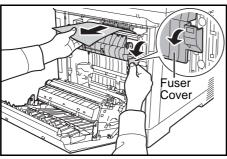
3 If a paper jam reaches the fuser unit as shown, open the fuser cover, grasp the paper, and pull it out.
